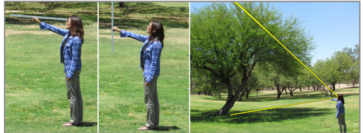
Figure 5. Stick method for measuring tree height. Use a portion of a stick or ruler that is equal to the distance from your hand to your eye.
